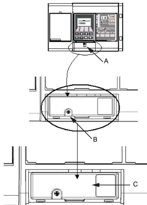
3. Pull out the air filter cartridge (C). This will stop the aspirator. If the aspirator does not stop, replace the filter switch.
