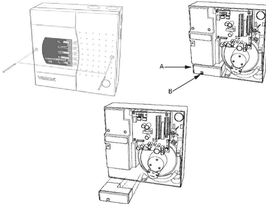
5. Insert a new air filter cartridge (A) (P/N: VSP-005).
